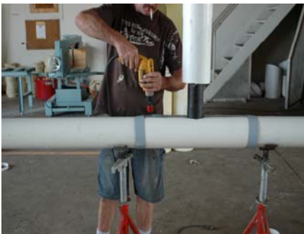
Drill 1" hole on each side for foam and apply tapecoat to seams
