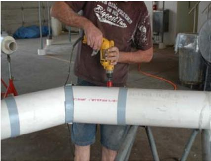
**Drill 1" hole on each side for foam**
